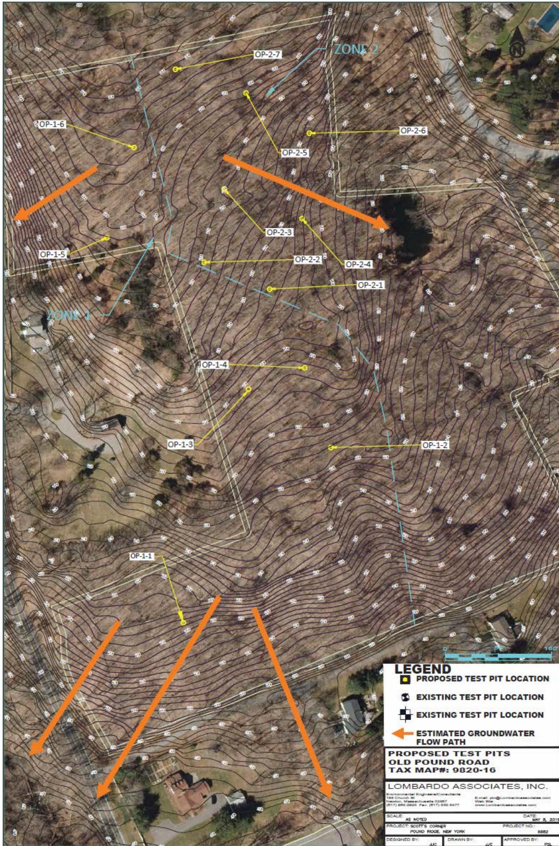
Figure 6-5-1 Old Pound Ridge, Test Pit Locations
