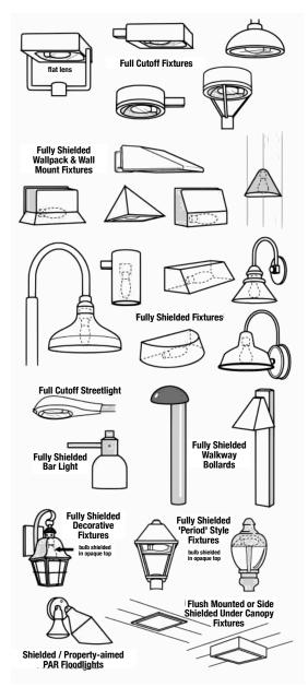
Examples of shielded light fixtures that shield the light source, minimize glare and light trespass, and facilitate better vision at night.
