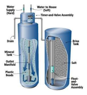
Figure 4.1: water softener system (www.appleplumbing.com)
