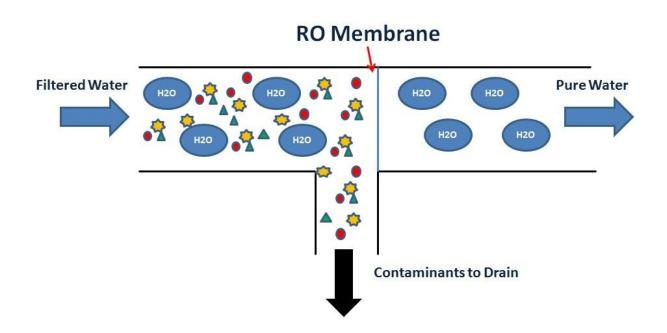
Figure 4.2: How a reverse osmosis water filter works (www.h2oavenue.com)
