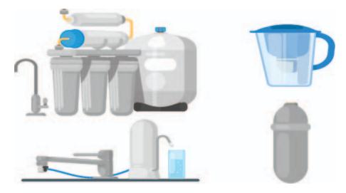
Examples of in-home drinking water filtration units. Top left to bottom right: RO tap unit, charcoal filter water pitcher, charcoal filter tap unit, and refrigerator water filter.
